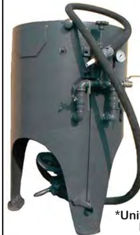
900lb. Pangborn w/electric remote controls & Thompson Valve for abrasive metering.
