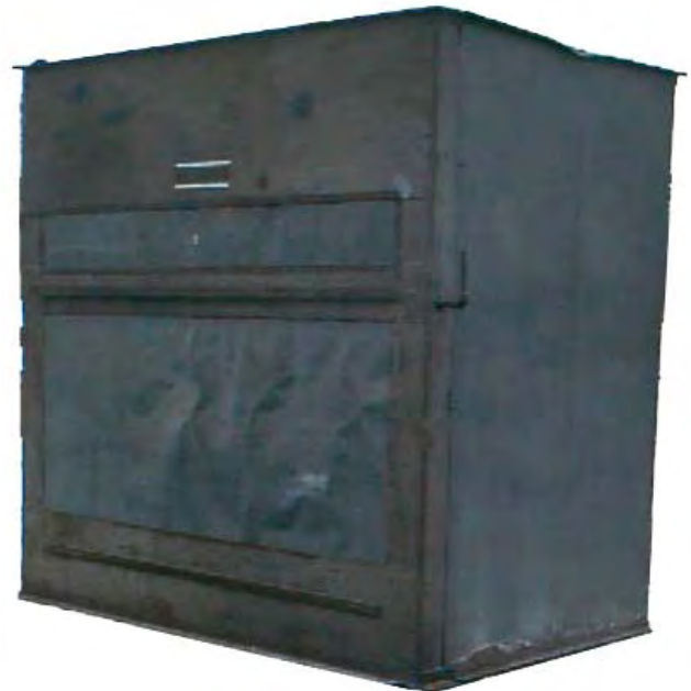
Steel blast room - size 7'-6" x 5 1/2" x 7 5-1/2" 4 walls, roof and door on one end
